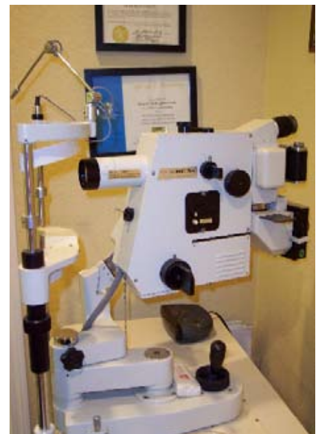
A retinal camera is used to photograph the back of the eye, including the retina. It is used to document eye diseases.
